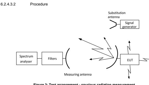
Figure 3: Test arrangement - spurious radiation measurement above 1 000 MHz for an EUT with antenna
