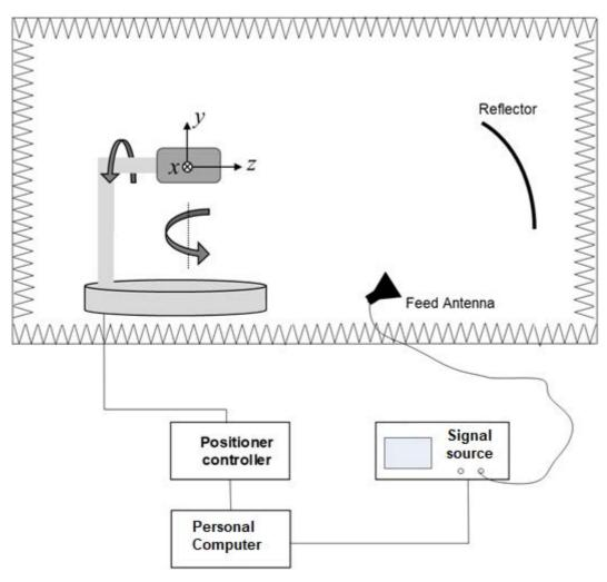
Figure B.5: IFF (CATR) measurement setup
