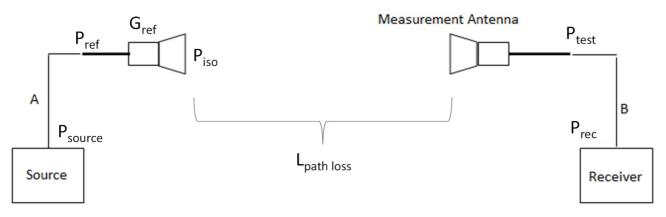
Figure B.8: NFTF - Typical setup for path loss measurement
