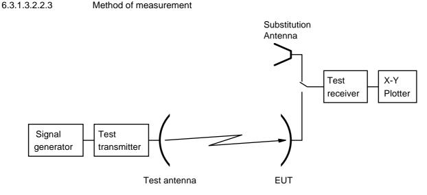
Figure 6: Test arrangement - antenna transmit gain measurement
