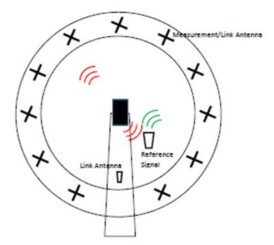
Figure B.7: Typical NFTF measurement setup
