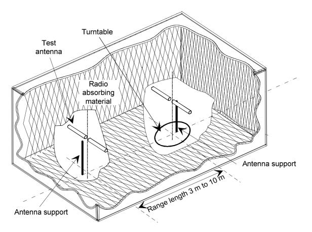
Figure B.1: A typical Anechoic Chamber
