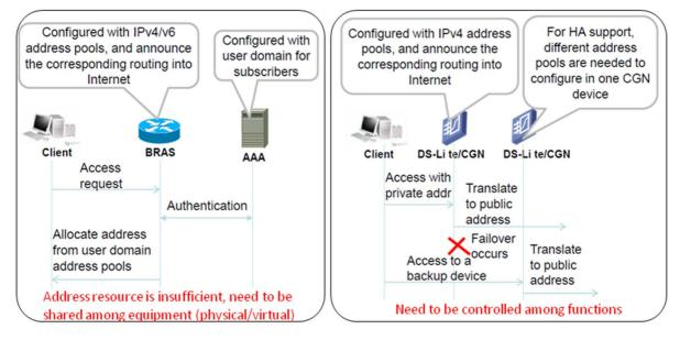
Figure 5-5: Current Problems in Operator IP Managed Networks
