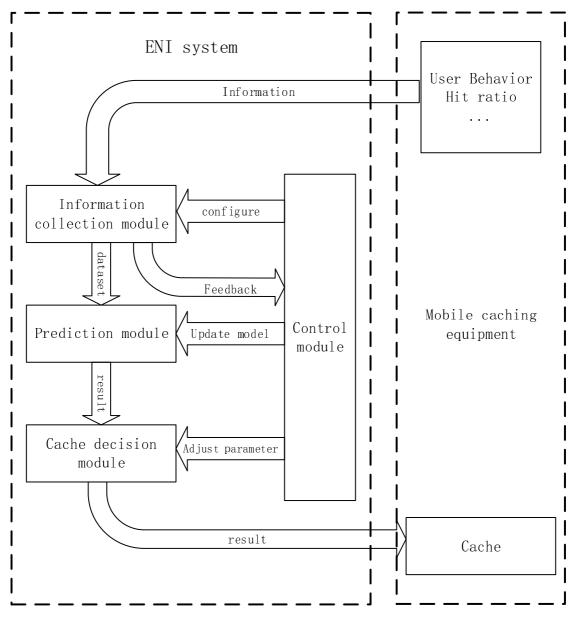
Figure 5-25: AI-based mobile caching
