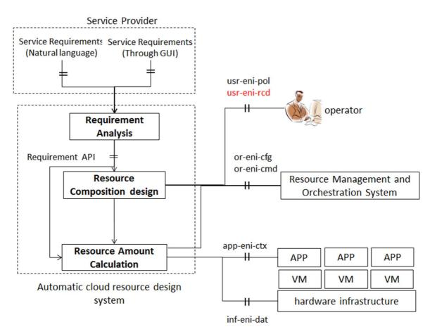
Figure 5-18: Automatic Cloud Resource Design System
