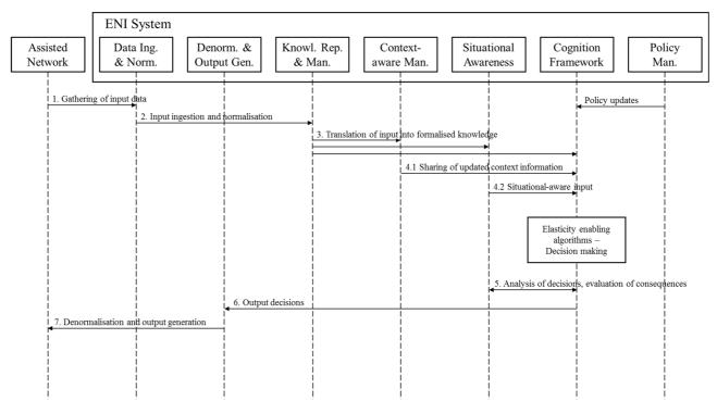
Figure 5-10: Example Flow of information among the ENI System's functional blocks and the Assisted System
