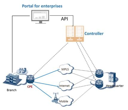
Figure 5-24: Intelligent carrier managed SD-WAN service
