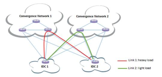
Figure 5-1: Policy-driven, automatic IDC traffic steering
