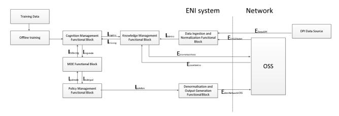
Figure 5-12: Mapping to ENI reference architecture for Application Characteristic based Network Operation For training data, it can be pre-prepared one or the one from OSS and DPI data Source.
