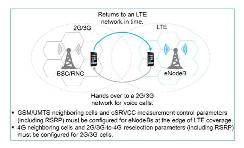
Figure 5-20: Interoperability between VoLTE and 2G and 3G
