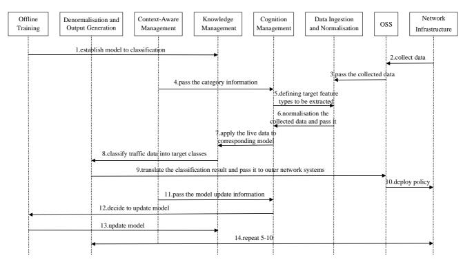
Figure 5-16: Scenario of AI enabled network traffic classification
