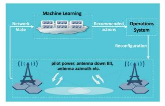
Figure 5-6: Coverage and Capacity Optimization
