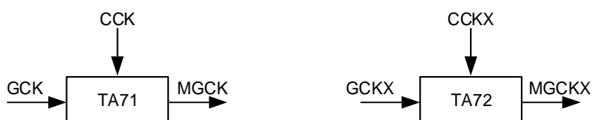
Figure 4.8: Generation of MGCK from GCK and CCK and MGCKX from GCKX and CCKX
